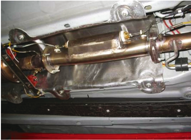
Fig. 8. The UV gas sensor mounted underneath the car
